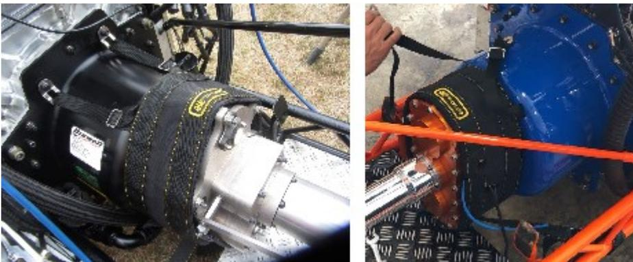
Because some **planetary gear transmissions behind a bellhousing** are very narrow a blanket is not a good option.
