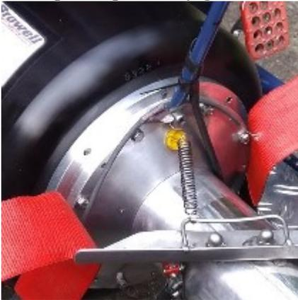
Example of internals of this transmission; Ring gear is stationary, Sun gears are driven by the Clutch and Gear in the middle is driving the shaft to the rear axle.
